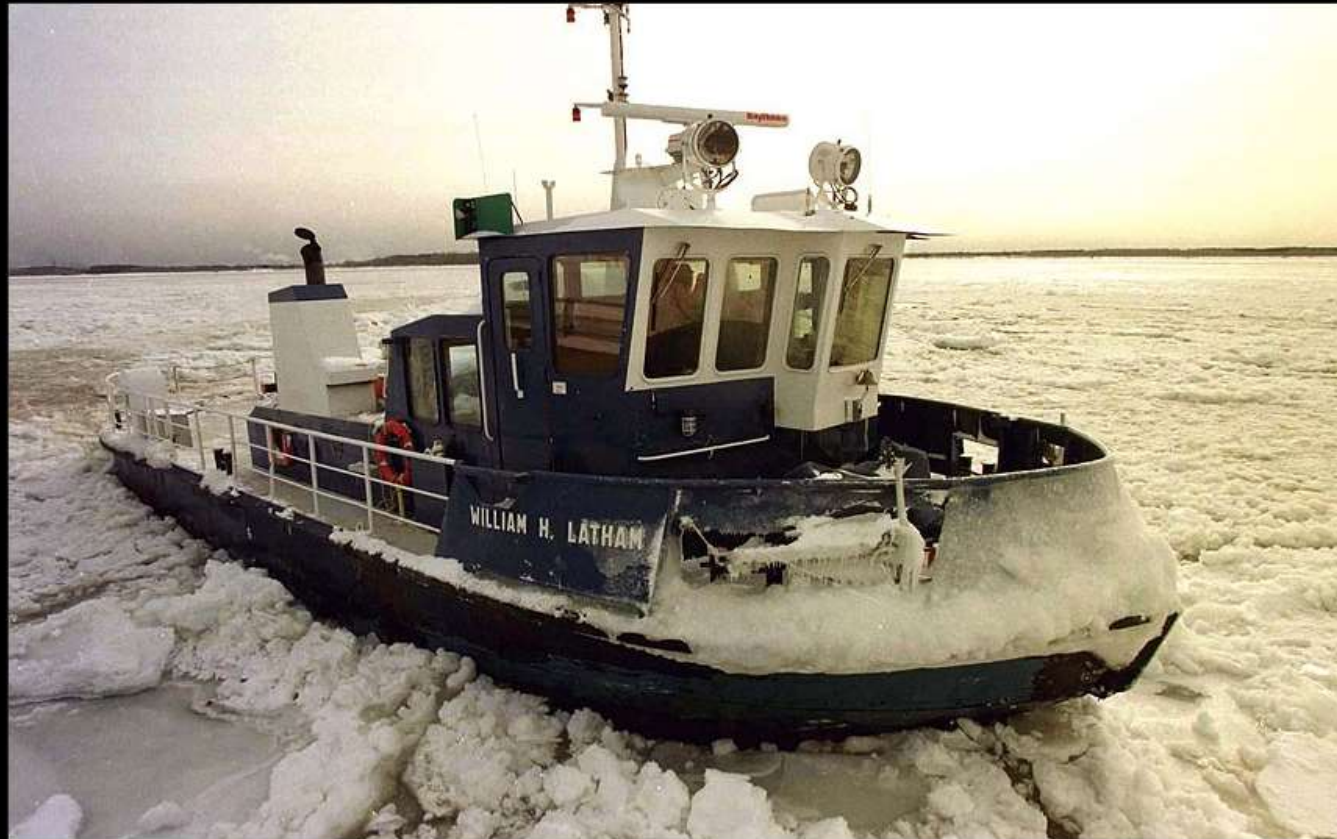
The ice cutter William H. Lathan navigates through thick ice in the Niagara River. The cutter works constantly in cold weather to keep the water intakes for the Niagara Falls hydro-electric plants free of damaging ice.
